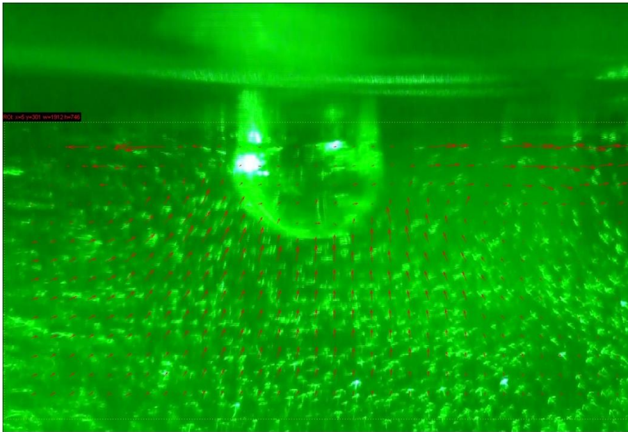
h) t = 0.6 s. The flow pattern is qualitatively similar to the previous two photographs. The average velocity of the field is 0.99750 mm/s.
