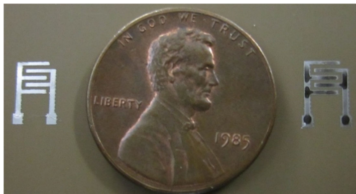
Figure 3.10 Inkjet printed silver electrodes during (right) and after complete (left) curing.
