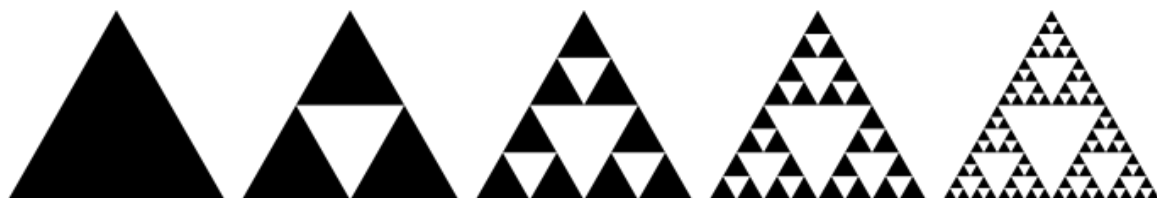
Figure A.2 Sierpinski triangle evolution in which each iteration removes one-quarter of the remaining area as a series of ever-smaller triangles. Four iterations are shown from left to right. [57]
