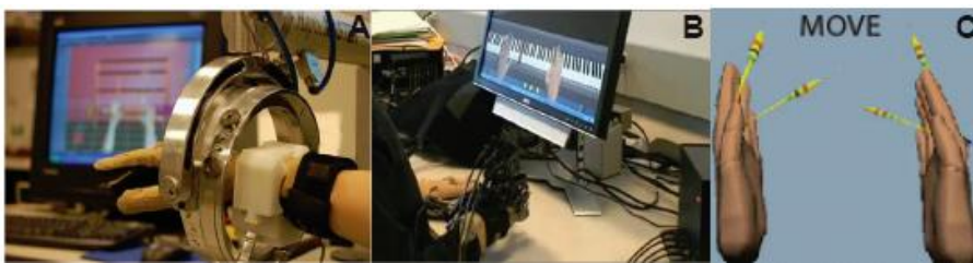
Figure 5.1 A. B. Robotic arm, data glove and force-reflecting hand system used in the VR therapy. C. VR feedback during the fMRI movement task.
