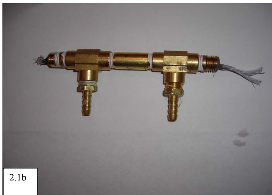
Figures 2.1 (a) Component parts of the membrane module (b) assembled module.
