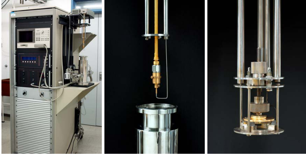
Figure 1.1 Dielectric Spectrometer with high and low-frequency attachments. Source: Institute of Solid State Research
