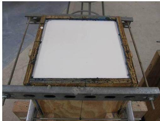
Figure 3.20 Application of hydro-stone ® gypsum cement.
