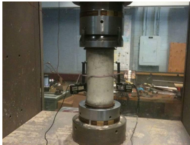
Figure 3.16 Measuring axial deformation of cylinder by a pair of extensometers.
