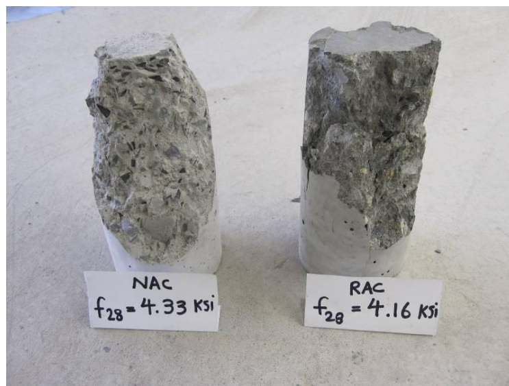
Figure 4.2 Typical failure of RAC and normal concrete cylinders.
