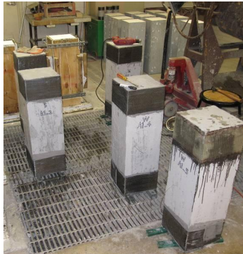
Figure 3.15 Additional end confinement using GFRP laminates.
