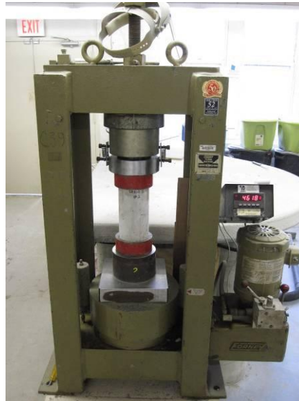
Figure 3.7 Testing machine used for measuring strength of concrete cylinders.
