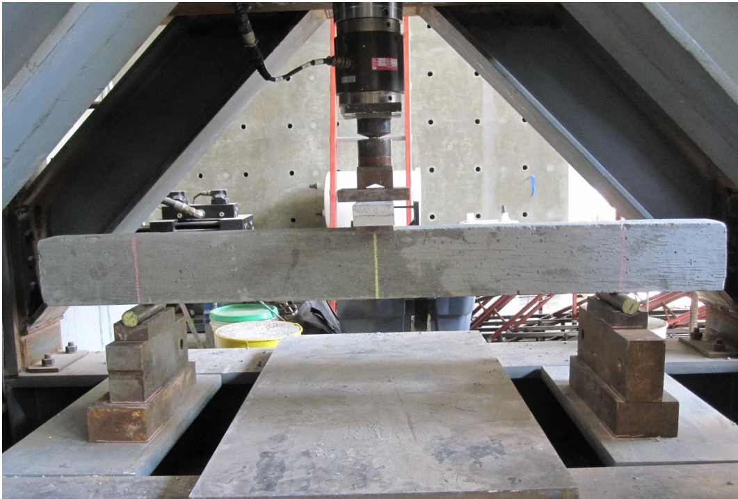
Figure 6.5 Beam test setup: (top) Beam-1, (bottom) Beam-2.
