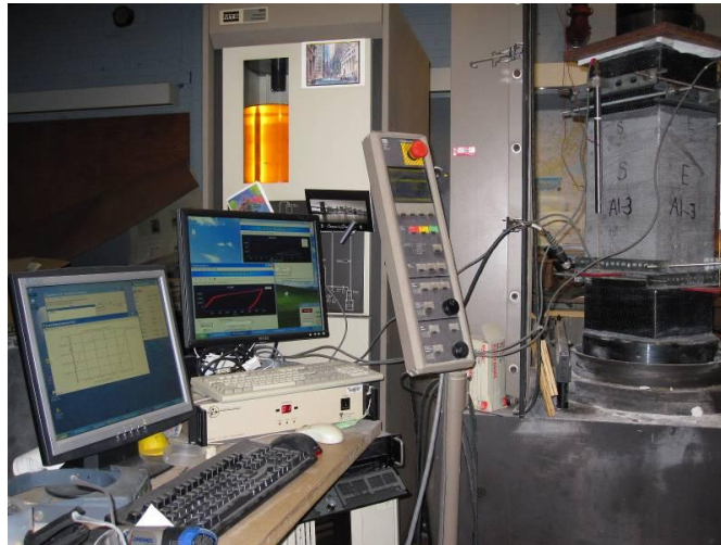
Figure 3.21 1000-kip MTS815 servo-hydraulic loading unit and other hardware.
