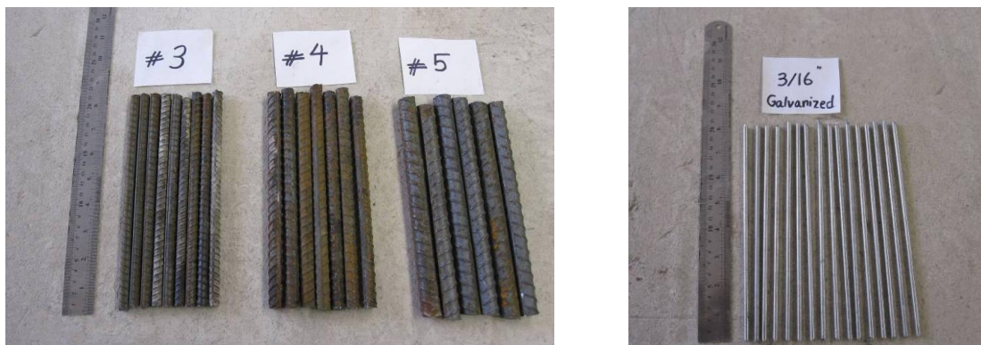
Figure 3.9 (left) Longitudinal rebar samples, (right) Tie steel samples.
