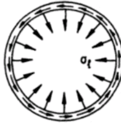
Figure 2.13 Confinement by circular spirals.
