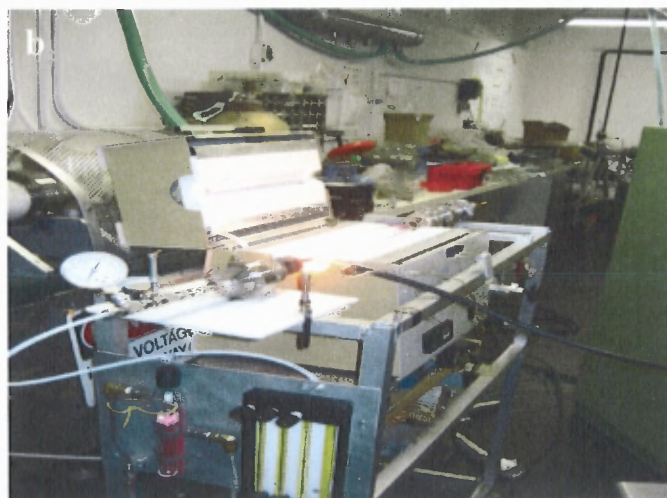
Figure 4.6 Experimental set-up for plasma-assisted synthesis: a) Schematic of Plasma-Enhanced Chemical Vapor Deposition (PECVD) apparatus, and b) Photograph of the PECVD set-up used in this work.
