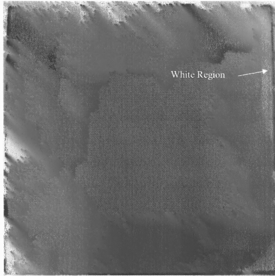
Figure 5.3 Photograph of back side of fired 125mm solar cell. On the bottom edge of the photograph, temperature non-uniformity can be seen at both corners.
