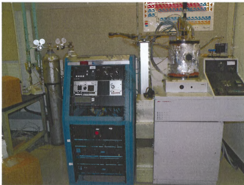
Figure 4.1 RF reactive magnetron sputtering system (Edwards Auto 306) at National Renewable Energy Laboratory.
