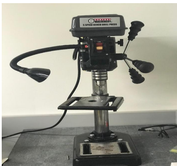
Figure 2.6 Drill machine for making inlet and outlet ports.
