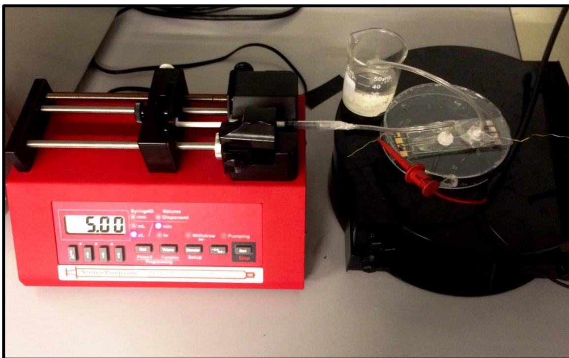
Figure 4.7 Experimental run for attachment of Anti Oxycodone mouse monoclonal antibody to functionalized CNT (in green) followed by Anti-mouse goat polyclonal antibody in a continuous process with 0.1x PBS solution
