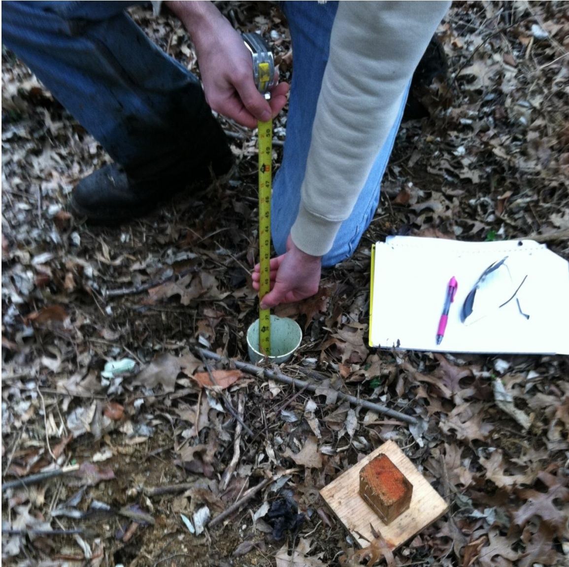
Figure 2.6 Reading water level from a monitoring well using a tape measure.
