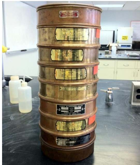
Figure 2.14 Sieve analysis set-up.
