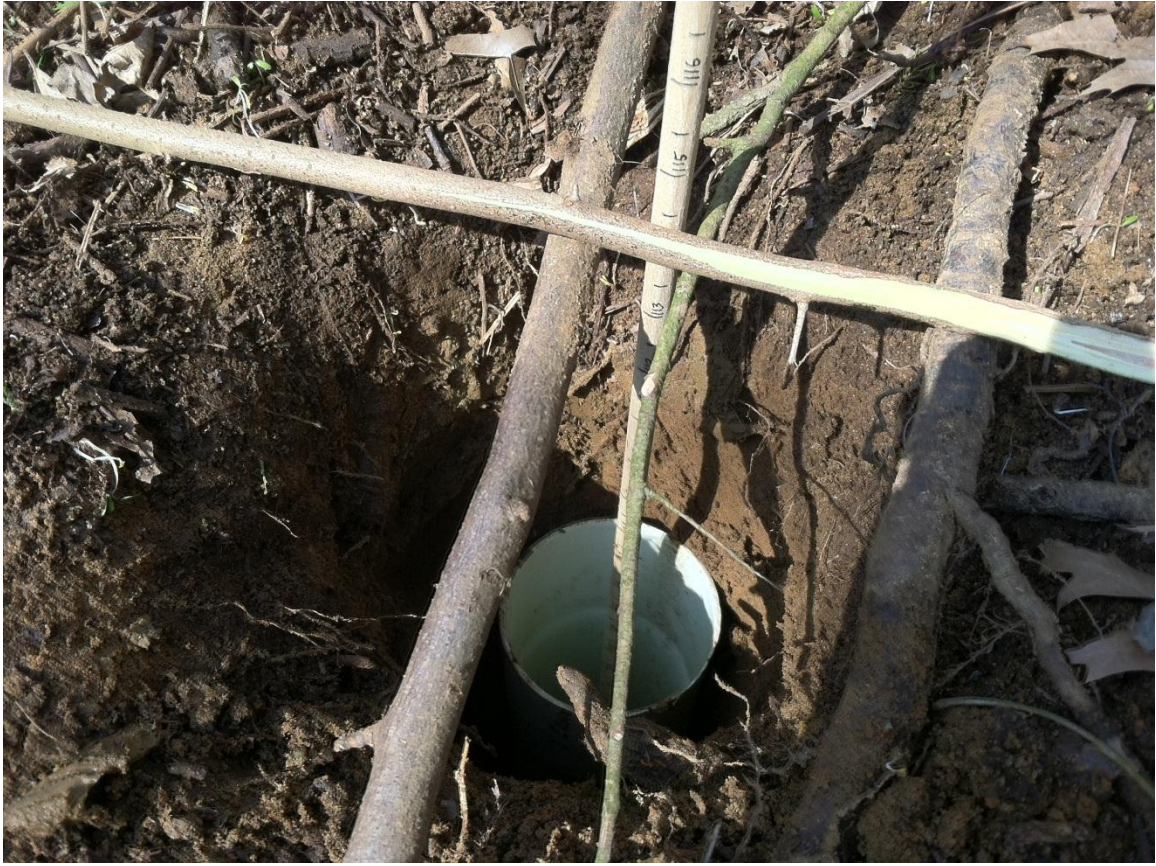
Figure 2.7 Reading water level from a monitoring well using a metered floating stick.
