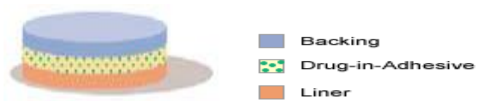
Figure 4.2 Diagram of a typical commercial nicotine patch [20]
