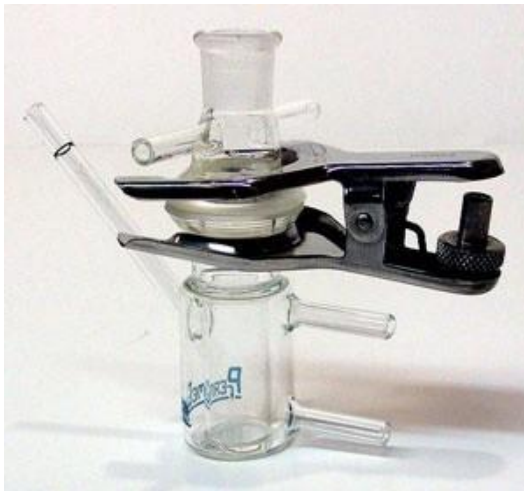
Figure 4.4 Fully assembled typical Franz static cell
