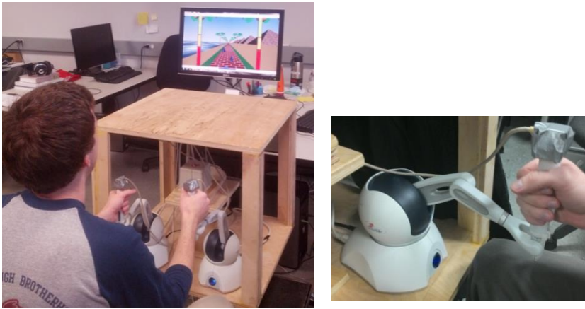
Figure 2.1 Experimental setup : (Left) A) VE monitor. B) NOB sensor on Phantom Omnis. (Right): Phantom device with NOB sensor.
