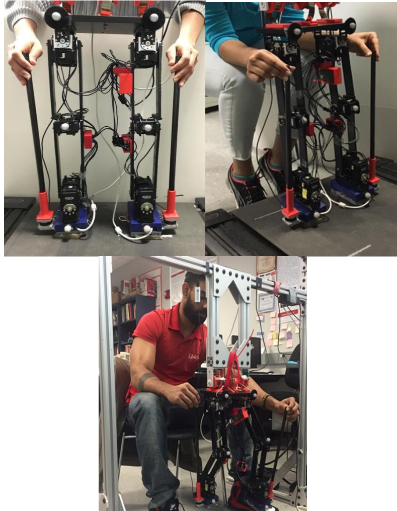
Figure 4.1 User control of biped a & b) User controlling the biped on treadmill. C) User controlling the biped in air during familiarization session.
