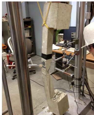
Column C1 at failure
