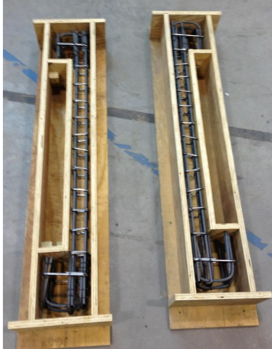
Figure 3.3 Wooden forms used for the test columns.
