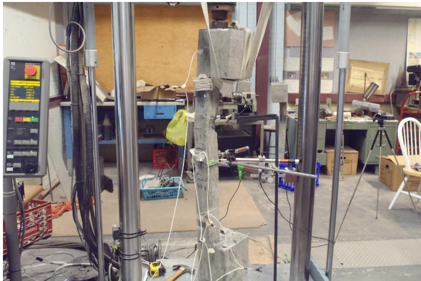
Column C6 at failure
