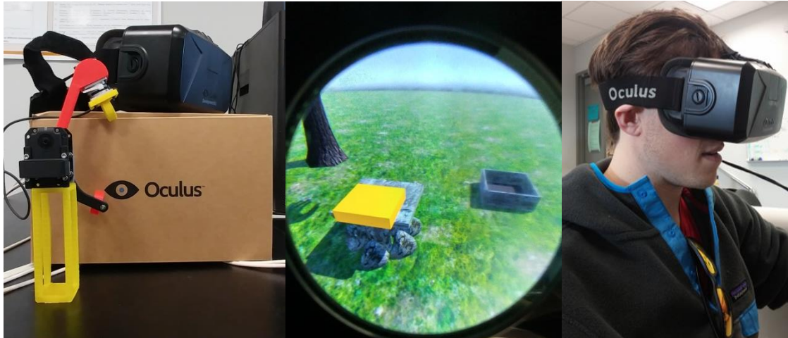
Figure 7.1. Left) Immersive VR components include the modular gripper and Oculus Rift. Middle) Stereoscopic view of virtual task viewed through Oculus Rift. Right) Individual engaged in immersive experience with visual and haptic feedback provided by Oculus.
