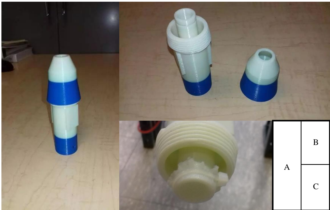
Figure 3.9 Receiver produced by 3-D printer.
