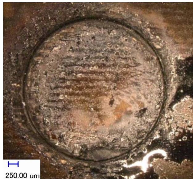
Figure 8 Initial laser drilling result (power: 900 W; speed: 10 mm/sec; single pass).
