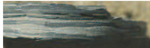
FIGURE 15. Facies D. Parallel-laminated shales with thin, very fine grained sandstone lenses forming connected starved ripples (Gaskill).
