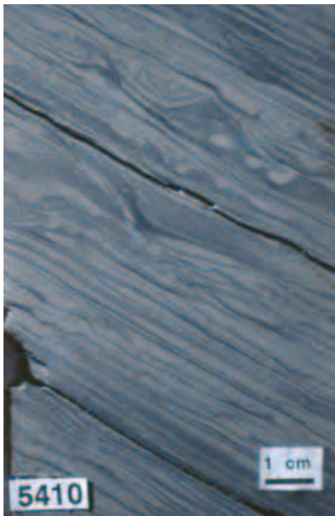
FIGURE 26. Facies F. Inclined strata with pseudonodules and ball and pillow structures (Fretz).
