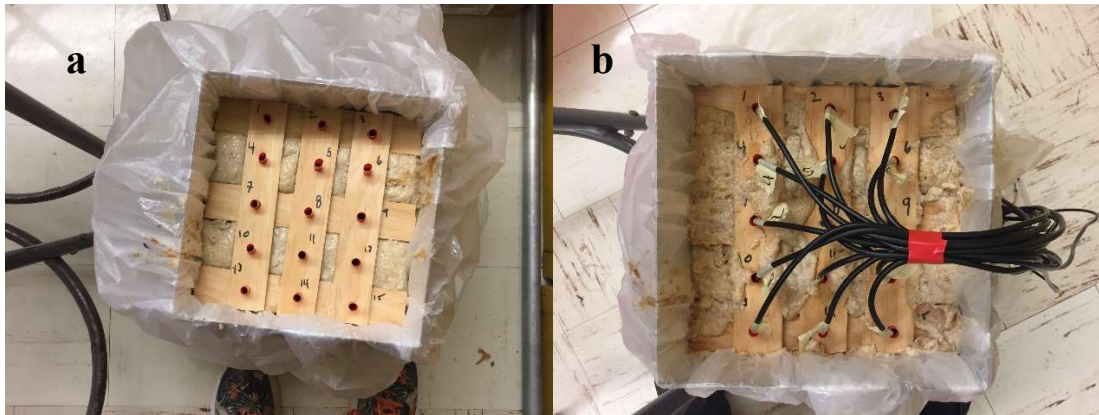
Figure 10: The sensor grid before (a) and after (b) the addition of the sensors.
