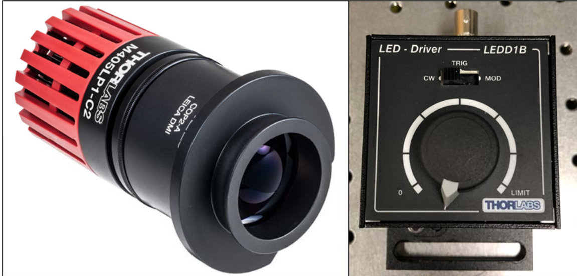
Figure 50. Left is a Thorlabs M405LP1-C2 LED. Source with center-wavelength 405nm and FWHM 12nm attached to a COP2-A collimating lens with Leica dovetail adapter. Right is the corresponding Thorlabs LED drive for this light source.
