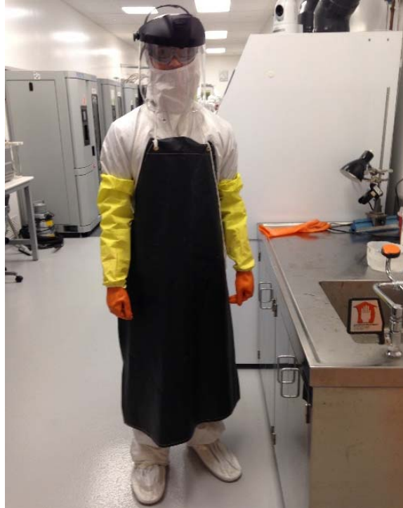
Figure 18. Cleanroom user with personal protective equipment (PPE). Standard PPE for acid work includes cleanroom gown, acid gloves, arm sleeves, chemical goggles, and face shield.
