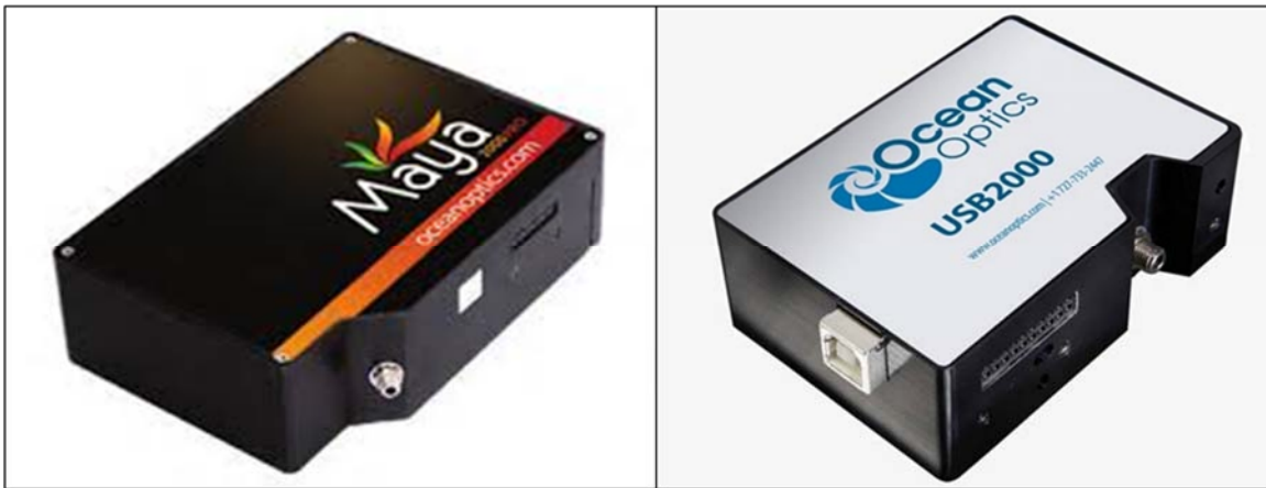
Figure 48. Spectrometers used for experiments. Ocean Optics Maya 2000PRO spectrometer (left) and an Ocean Optics USB2000 spectrometer (right). The spectrometers were used for recording different experiments' spectra.
