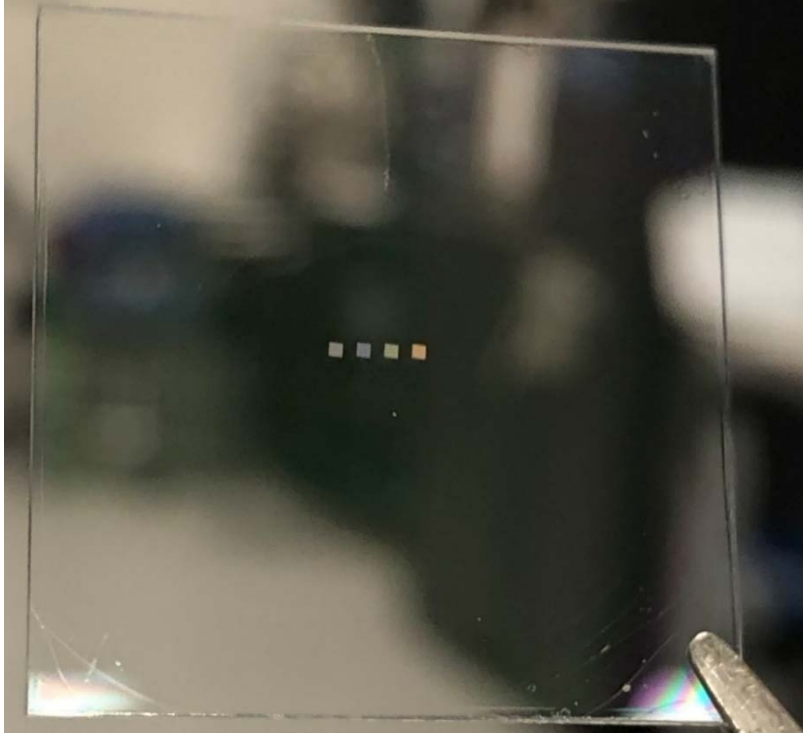
Figure 90. Arrays of bullseyes. Left to right, gap sizes 600nm, 500nm, 400nm, and 300nm.
