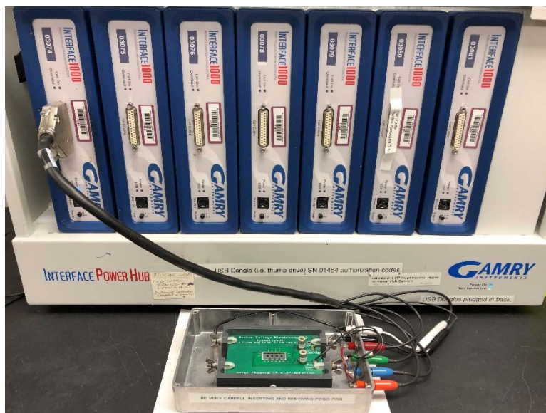
Figure 20. Gamry Instruments Potentiostat/Galvanostat Interface. Shown with reusable well apparatus and sample electronics interface for testing electrochemical experimentation.
