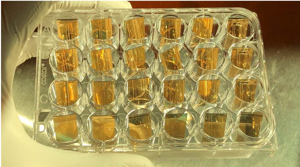
Figure 44. Au on glass. Samples made for use with the BioNavis Navi200 SPR system.
