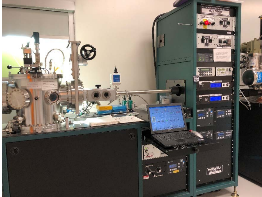
Figure 10. AJA International Sputter Deposition system
