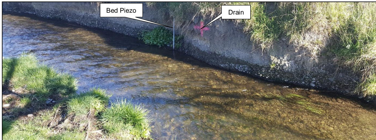
Figure 2-4 Flow Gauging Cross Section at Lower Beach Road. Pink Spray Paint on the Far Bank Indicates the Location of the Peg for Flow Gauging Use
