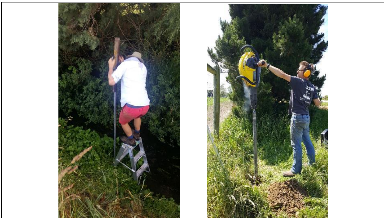
Figure 2-2 Environment Canterbury Science Technician Tom Johns Installing Piezo Boundary Bed (Left) and Poplar Bank (Right)
