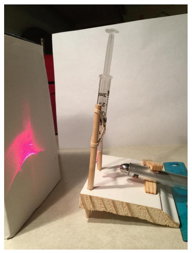
Figure 3 Side view of assembled microscope.
