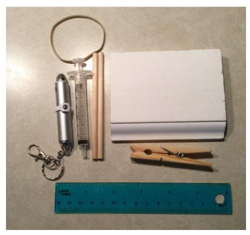
Figure 1 Parts for Liquid Drop Microscope with a 6" ruler for scale.
