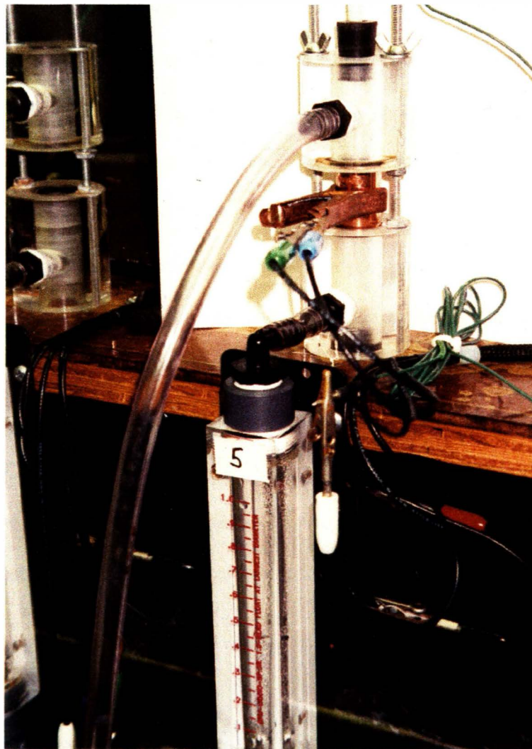
Figure 3-2: Reiber corrosion test cell.
