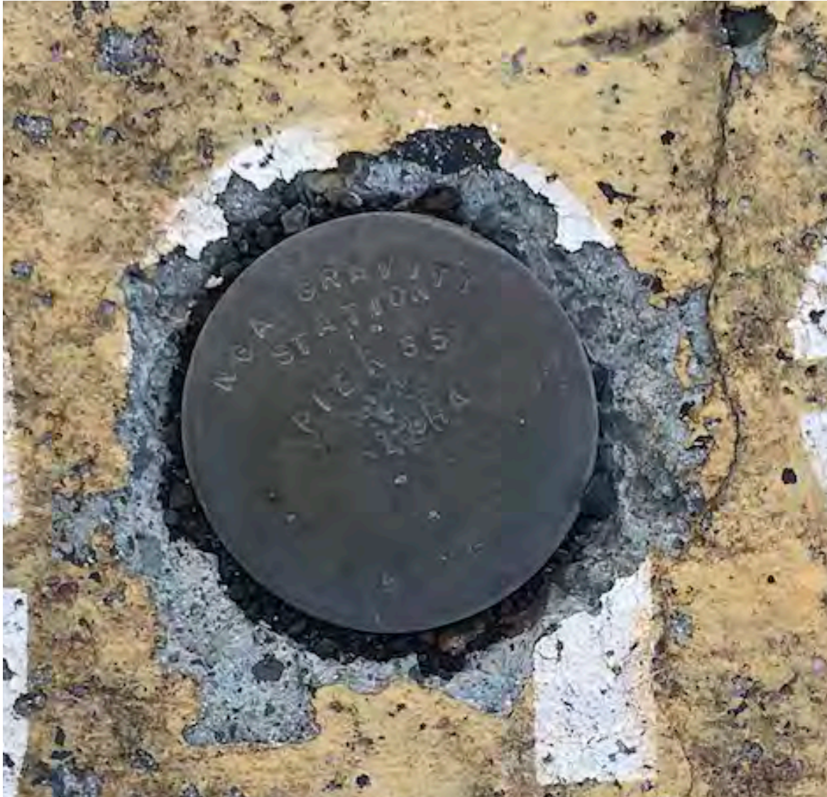
Figure D.7. Gravity station monument at Pier 35, Honolulu, HI that corresponds to the station description in Fig. D.6.
