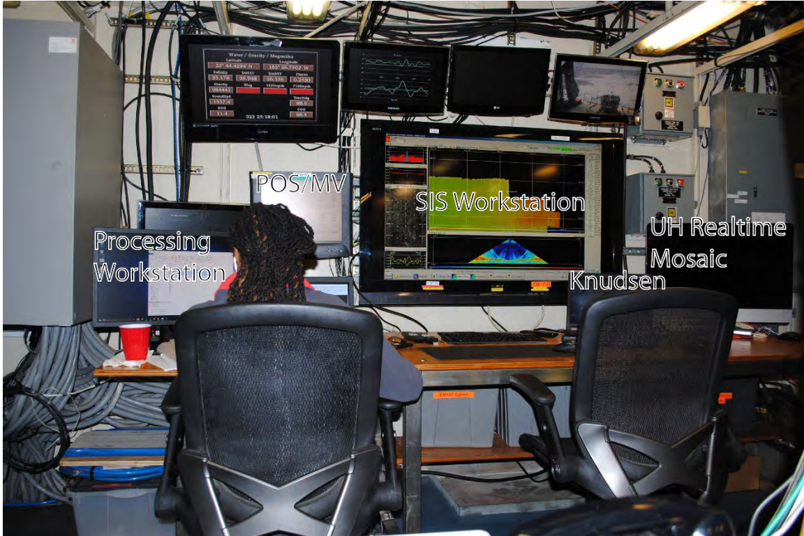
Figure 2.1: Instrument displays in the main lab of the RV Kilo Moana during KM1811. The large center screen is used for SIS, and the screen to the left displays the POS/MV real-time performance metrics, while the laptop to the right was used for Knudsen display. The laptop to the left was used for data processing and quality control. A separate real-time data mosaic service (far right) that was tested but not used for survey purposes was provided by University of Hawai'i.
