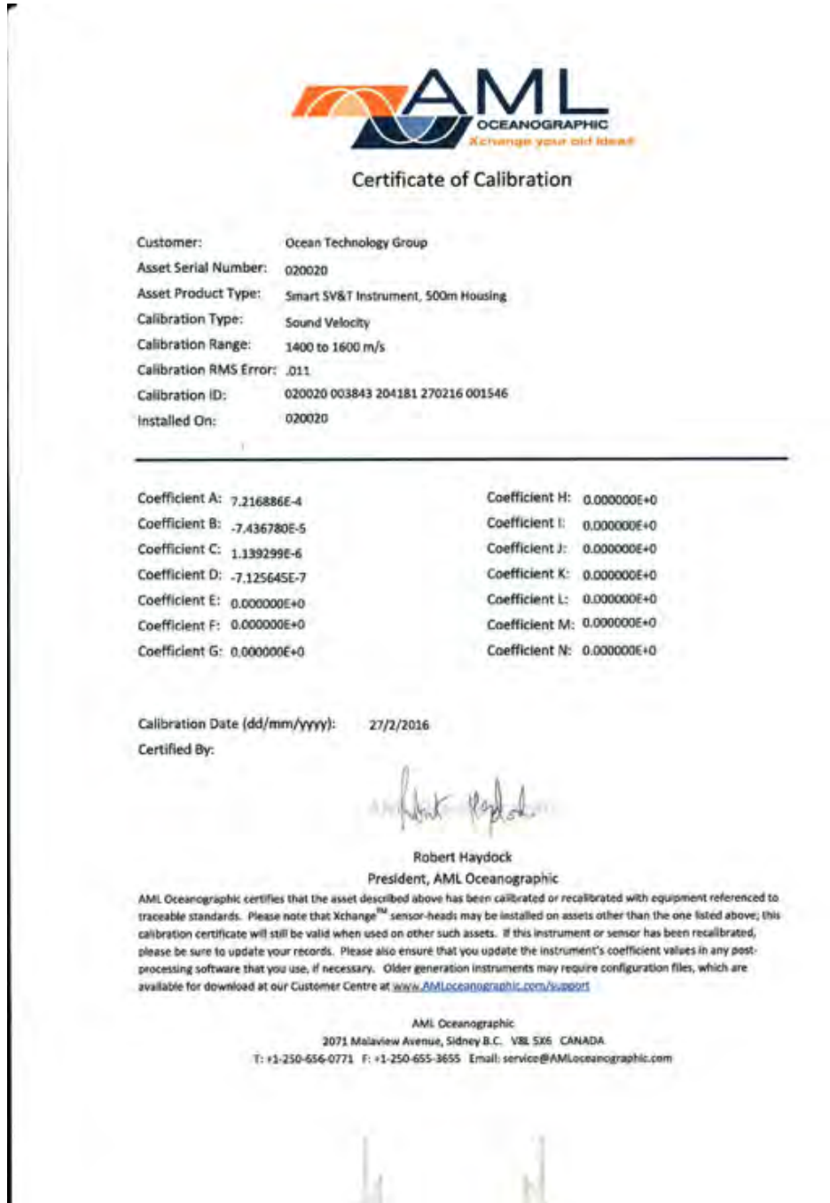
Figure D.3. Certificate of calibration for AML Oceanographic SV&T sound-velocity sensor.
