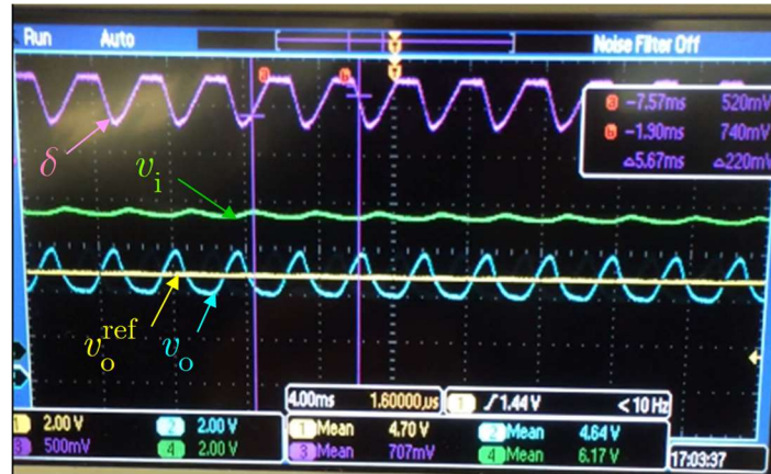
Figure 3.18 : Unstable condition due to an additional input filter
