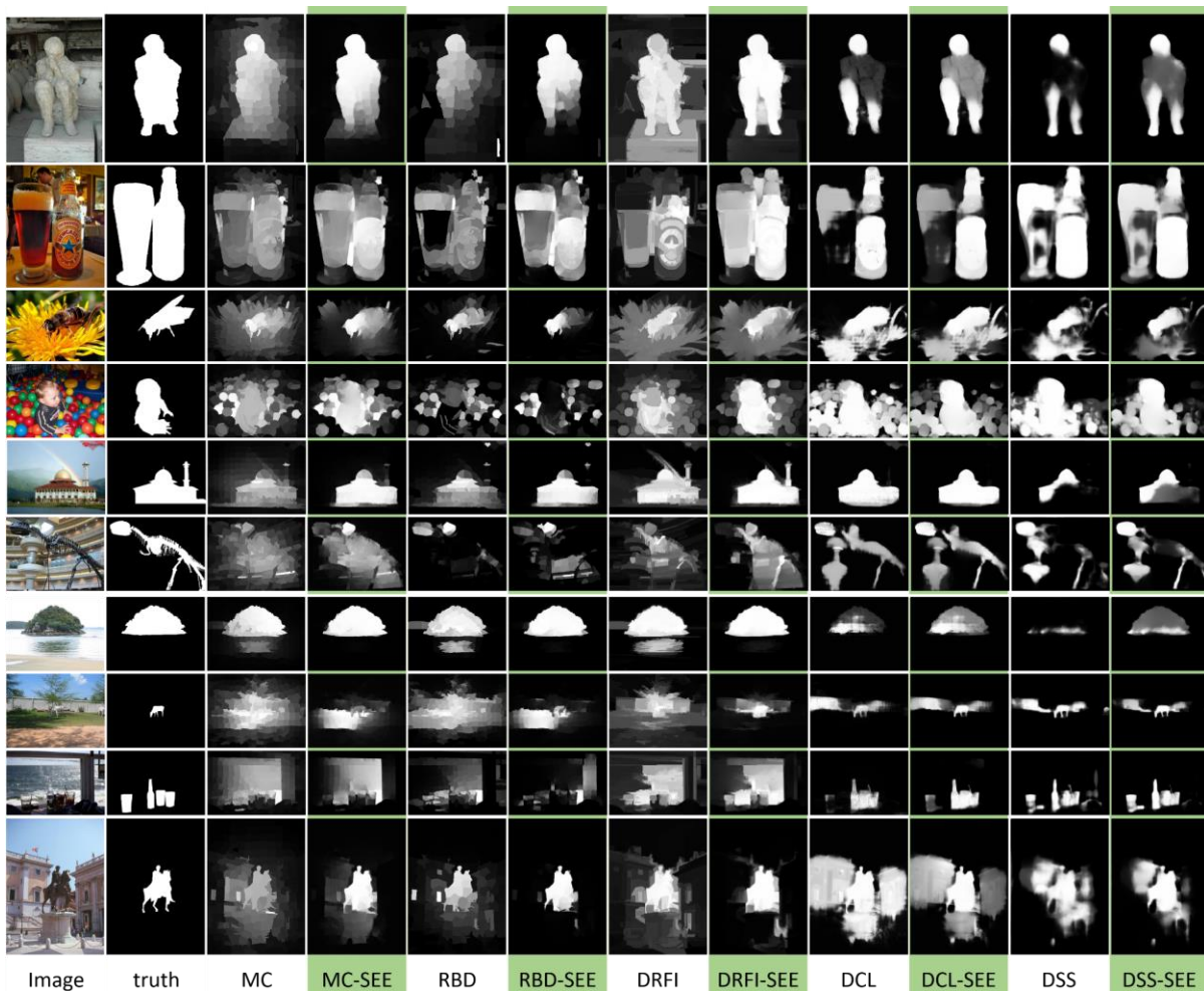
Figure 6-7 : Comparison of the results from 5 different SoA methods (MC, RBD, DRFI, DCL, and DSS) and their improvement using our SEE algorithm highlighted in green. The examples are chosen as some of the most difficult images in the datasets.
