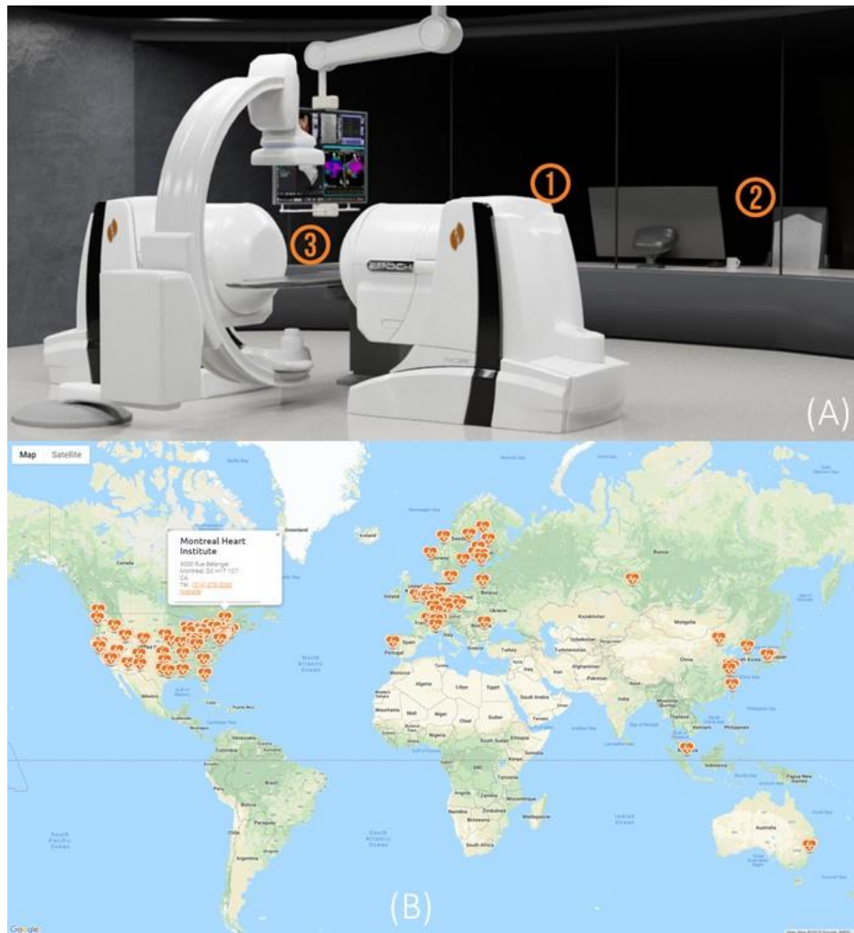
Figure 2.9 (A) Niobe Stereotaxis 1- remote magnetic navigation system 2- the workstation 3- the working zone of the catheterization (B) the location of the hospitals that have installed this system (source: http://www.roboticep.com/ )
