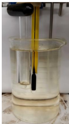
Figure A2. Boiling point of LPE and BPE additives, measured by the capillary tube method.
