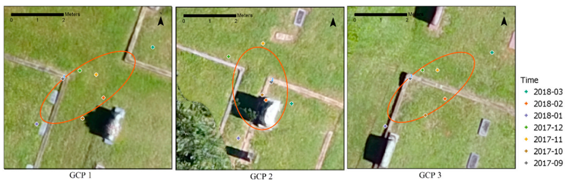
Figure 3. Positions of a GCP based on seven orthomosaics with the standard deviational ellipse of each positional cluster of a GCP.
