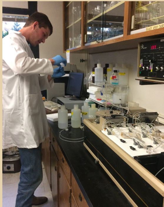
Jacob analyzes nitrate-N concentrations of pond water samples in the laboratory.
