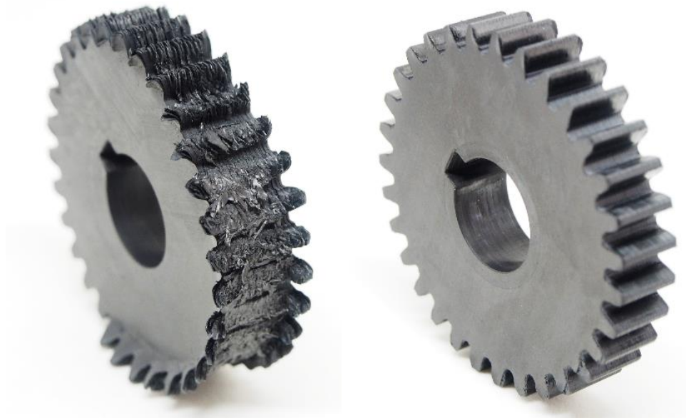
Figure 12: Damage of the PG Gear (left), raw Gear (right)
