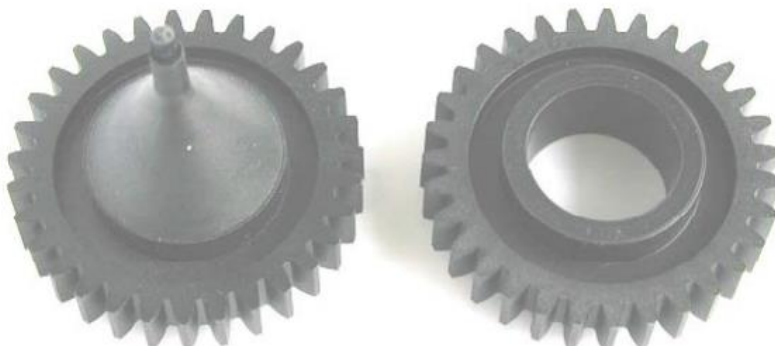
Figure 2: Injection molded gear blank (left) and finished test gear (right)
