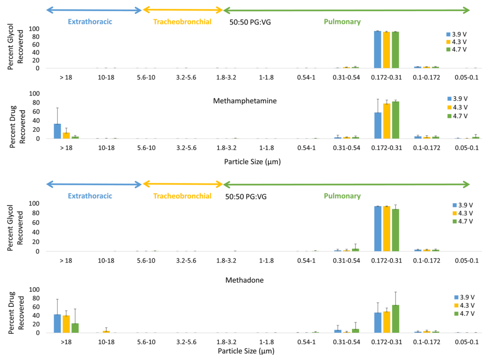
Figure 3. Particle size distribution of glycol, methamphetamine, and methadone by voltage at 1.8 \Omega .
