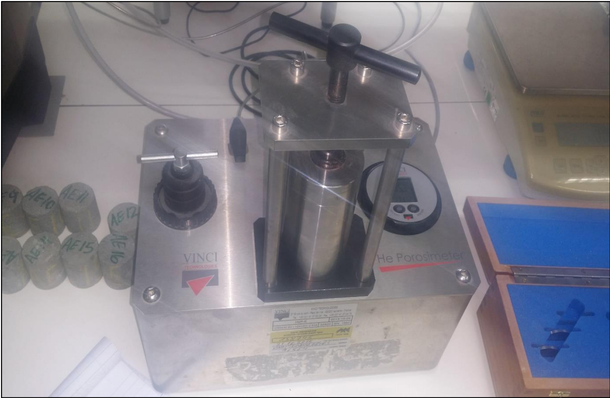
Figure 4-5: Porosimeter instrument used to measure the porosity of the core plugs.
