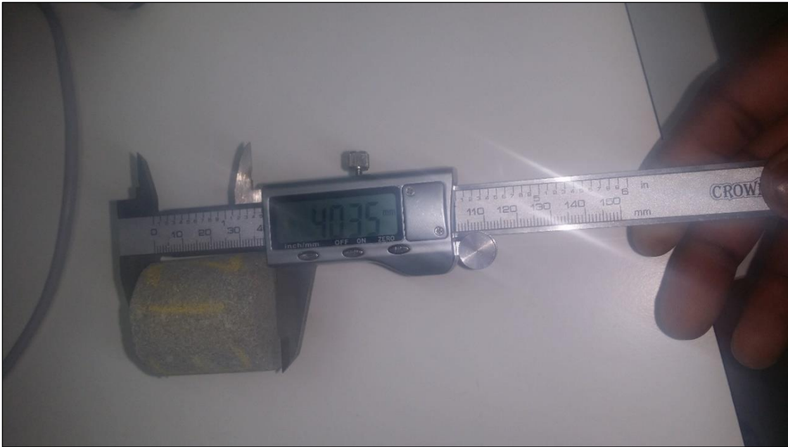
Figure 4-3: Calliper scale measuring the length and the diameter of the core plug.
