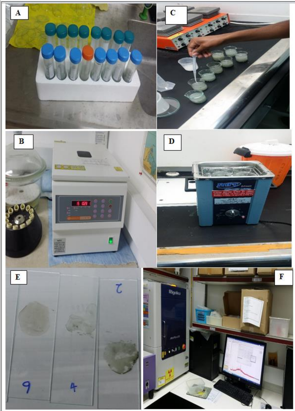
Figure 6-2: Illustration of the clay sample preparation for XRD analysis.
