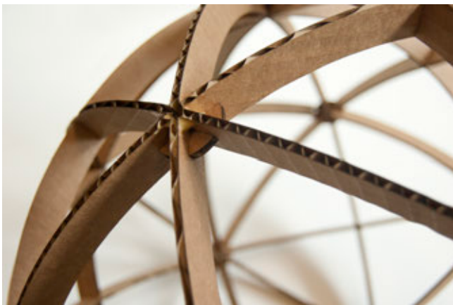
Figure 6. The first complete spherical shell, requiring glue to compensate for weak joints and mathematical error.
