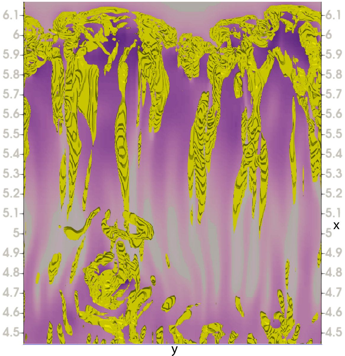
Figure 4.13: Top view of an isosurface of \lambda_{ci} = 3 of coarse-resolution DNS for the current at t = 12 . Near-wall structures are located between z = 0 and 0.1 . The streamwise velocity contours are at z = 0.03 .
