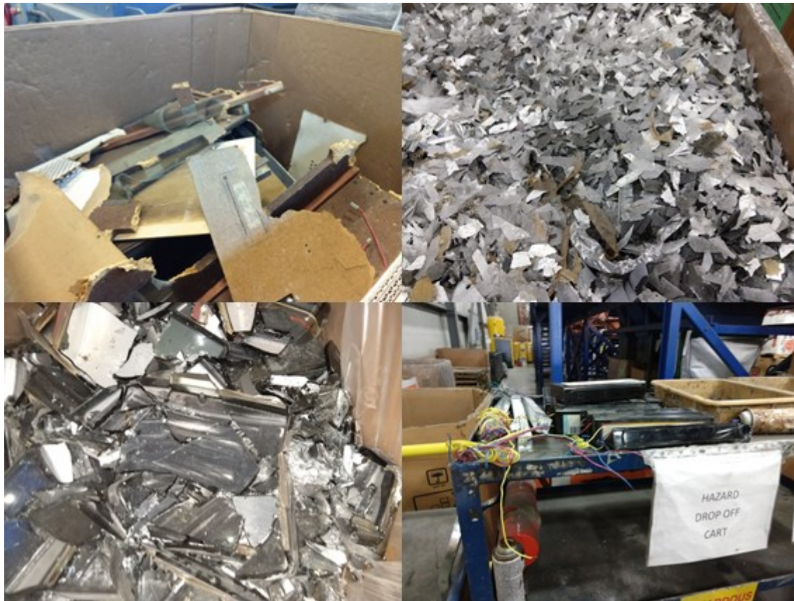
Figure 6 Starting Top Left Moving Clockwise: Wood Waste from CRT Display Processing, Thin Film Plastics from Flatscreen Display Processing, Panel Glass from CRT Display Processing, Hazards Taken from all Processes, all examples of items that incur downstream processing costs to the primary processor
