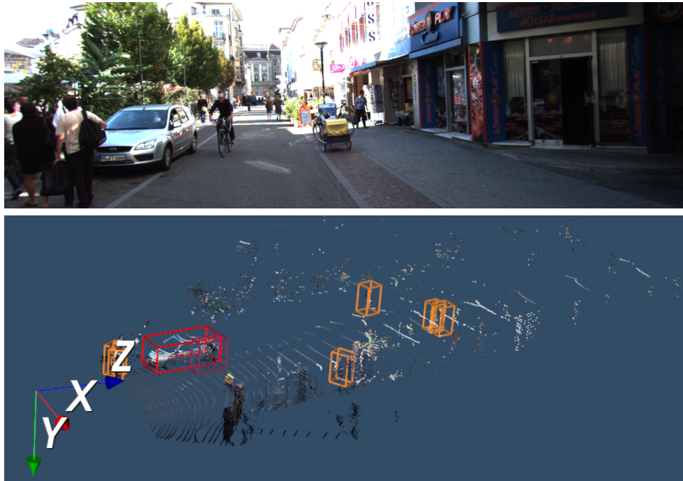
Figure 1.1: KITTI 2D image and LiDAR point cloud. Part of the data provided for the KITTI 3D Object Detection benchmark challenge [24]. Image colours are projected onto the point cloud. 3D bounding boxes are shown for vehicles (red), pedestrians (orange), and cyclists (burgundy).
