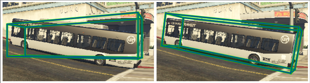
Figure 2.9: On steep slopes vehicles appear out of their ground truth 3D bounding boxes using the KITTI data format (left), but the PreSIL augmented annotations correct this problem (right).
