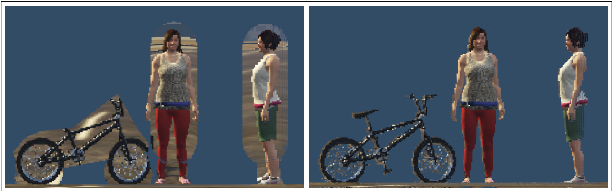
Figure 2.4: Image colors projected onto a point cloud display the difference between ray casting (left) and the PreSIL point cloud generation method (right) with a view of pedestrians and a bicycle. Note: For display purposes a higher LiDAR resolution was used for this graphic.
