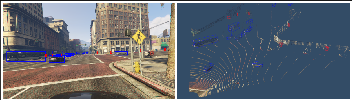
Figure 2.1: Annotated image and point cloud pair from the PreSIL dataset
