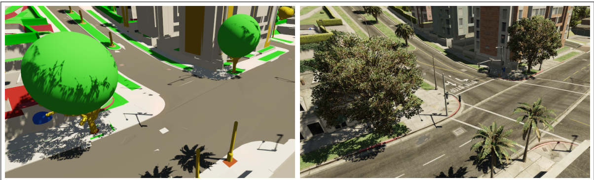
Figure 2.2: Collision meshes simplify physics calculations. A screenshot from GTA V shows the difference between the collision meshes (left) and the final rendering (right).
