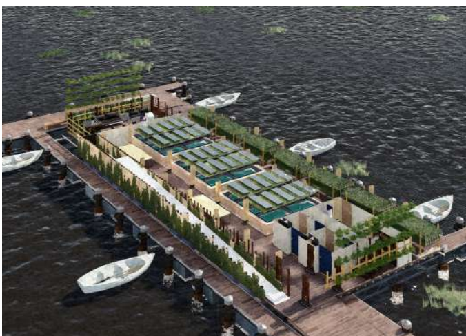
FIGURE 4.24 1st floor highlighting the Aquaponic grow beds over the fish tanks as well as those on the south side of the building
