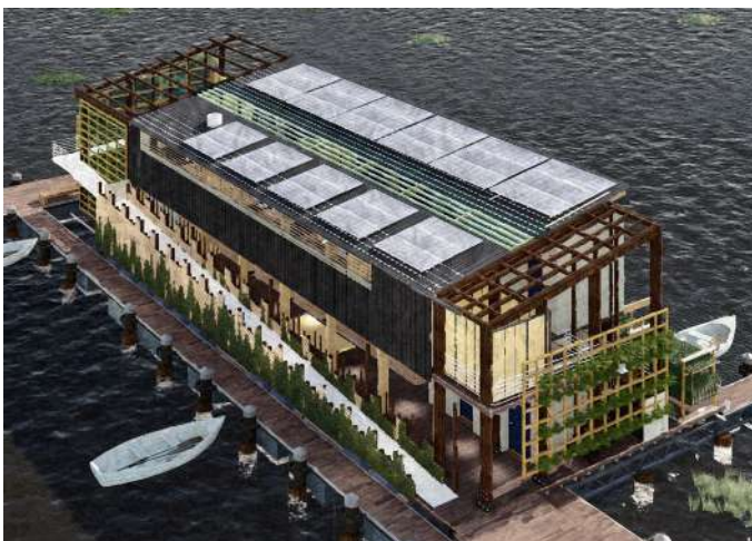
FIGURE 4.31 P.V solar panels installed on the roof to supply electricity primarily to the Mechanical room and also act as a back supply of electricity for the rest of the building
