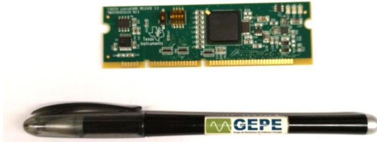
Figura 5.20. DSP TMS320F28335, *Texas Instruments*.
