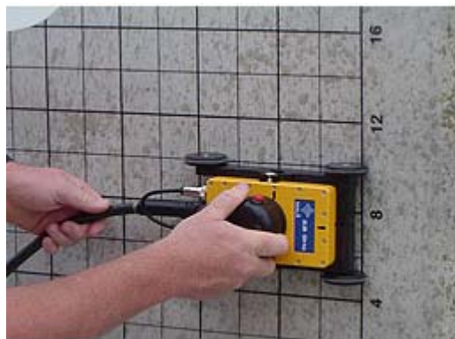
Figure 24. Example of monostatic GPR unit ( http://www.betagrouppgc.com/services.html )
