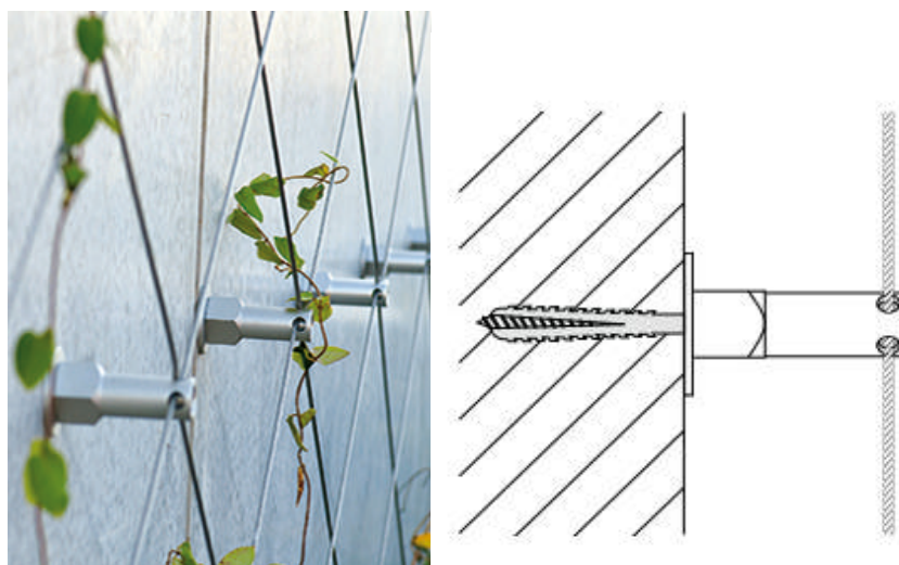
Figure 49.Greencable system Construction detail
