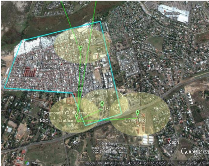
Figure 1: Project office within Masiphumelele township. Green lines represent TVWS/5GHz WiFi hybrid backhaul links are shown in green, yellow circles are 2.4 GHz WiFi hotspots.
