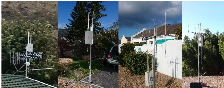
Figure 2: Outdoor measurements setup: (a) Static installation on roof (b, c) Mobile installation 500m up the road (d) Mobile installation 2.2 km away behind a tree
