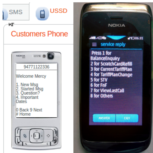
Figure 2: Left: Example Maternal Health USSD application running on IdeaMart USSD Simulator; Right: USSD home screen for Indian mobile operator BSNL.
