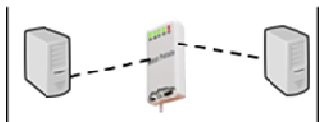
Figure 3: Scenario 2 (2Hop), one meter distance between the left Unix box and the MP. 15 Meters between the MP and the Unix boxes.
