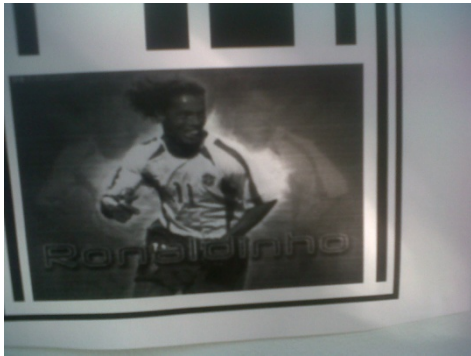
Figure 7 - An example of a poorly taken image. Notice how the left guidebar is not in the frame, thereby causing the algorithm to fail.
