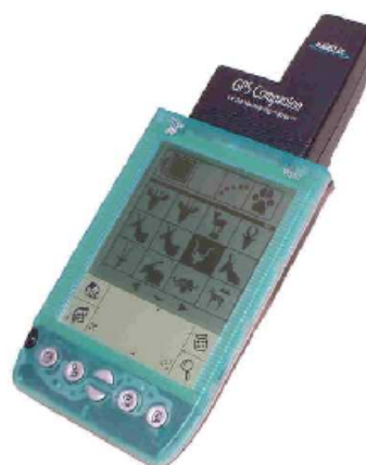
Figure 6. The latest hardware for the Field Computer: Handspring's Visor. Attached to the expansion port is the Magellan GPS Companion, a 12-channel global positioning system receiver.
