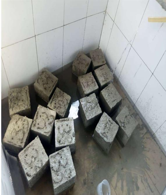
Plate VI: Cube in the curing tank
