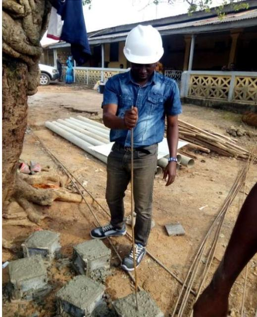
Plate I: Compacting of concrete in layers.
