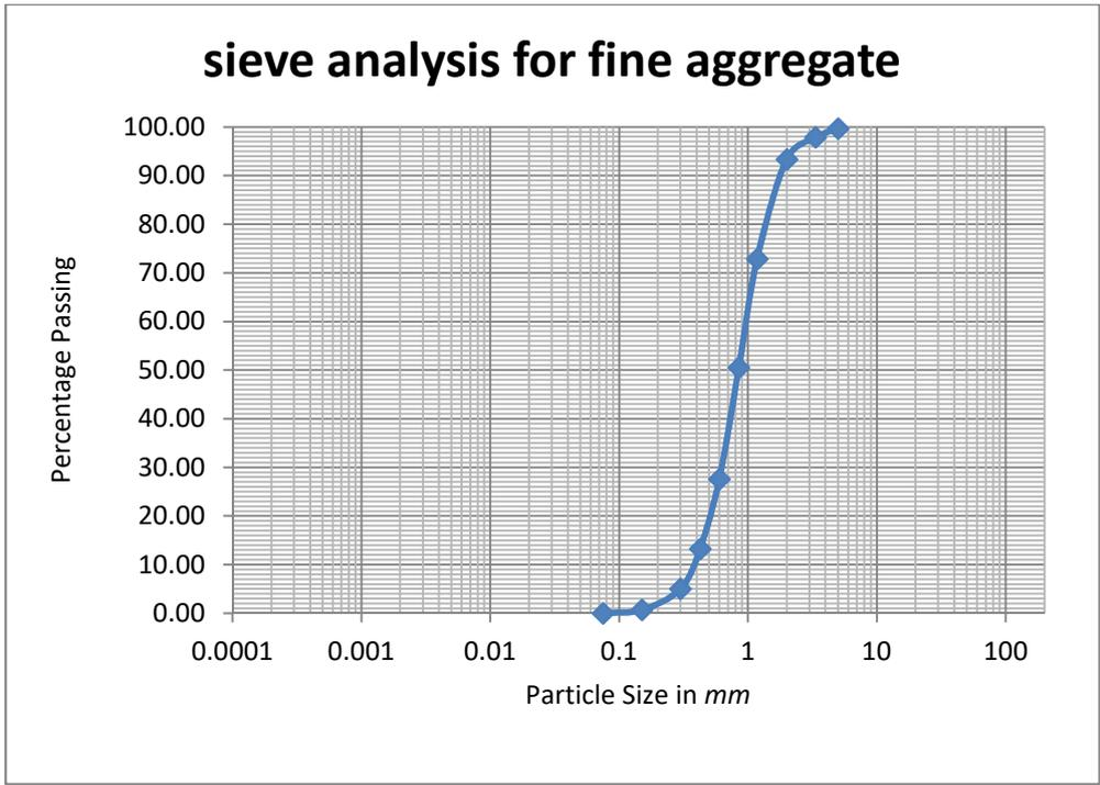
**Figure 1: Particle- Size Distribution Curve for Sand**
